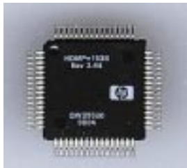
1.25Gb/s Gigabit Ethernet Transceiver <$6 in volume (datacom application)
