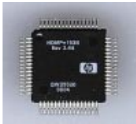
1.25Gb/s Gigabit Ethernet Transceiver <$10 in volume (datacom application)
